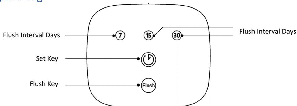
**Power first supplied:** system beeping meanwhile lights are flashing, with the five lights flashing simultaneously for one time, system enter the factory default setting(15 days), if there is no other operation, system enters sleep mode in 8 seconds.
